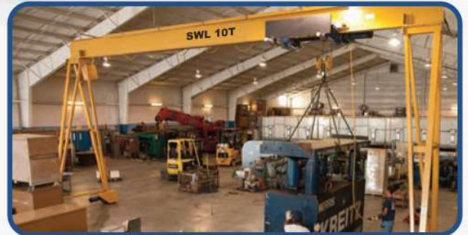
A 10-Ton Verkrönn PS Gantry Crane with power drive using guide angle for easy travel over a fixed route.
