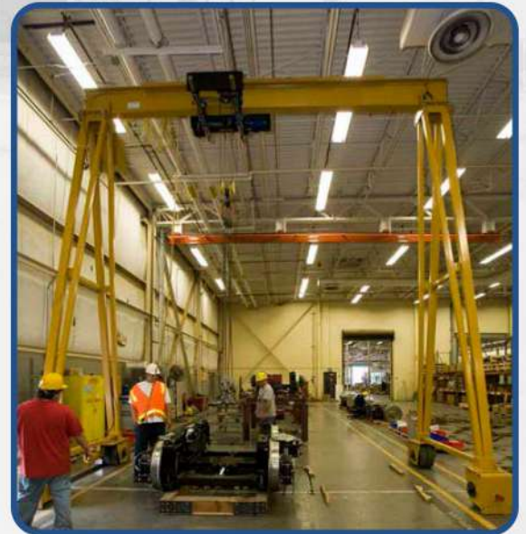
A 7.5-ton PS Gantry Crane with a Verkrönn Guide Angle Power Drive Kit & Guide Rollers for high volume, high capacity travel along a fixed path.
