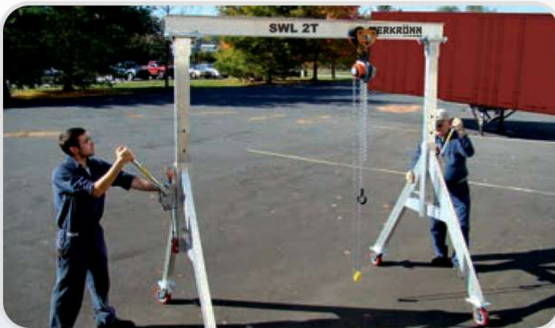
Two workers adjusting the height on an aluminium gantry crane using a Lug-All Winch Hoist.
